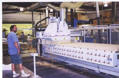
A pneumatic lift has been installed between the company's two Weeke CNC machining centers. Either operator can easily lift a panel from a stack and set it into place on his machine.
